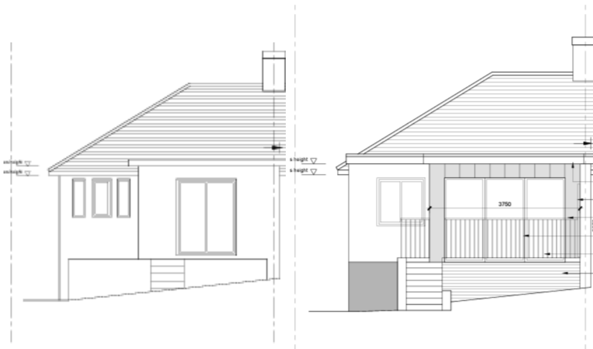
Figure 3: Pre-existing and existing rear elevation:
